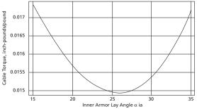
The actual computation of cable torque under load is a complicated problem as when the angles of inner and outer armor are changed, the tension carried by each layer and the torque are changing.
