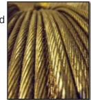
When a new cable is spooled onto a shipping reel and therefore not under significant tension, the additional space may accumulate between one or two wires giving the appearance of a wide gap in the armor. This effect is further accentuated when protective grease is applied and accumulates in these gaps. This is a normal condition and the gaps will equalize once installed and normalized during field operations.
