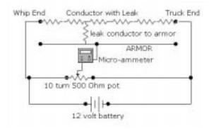
Remember before any type of leak location procedure is started be sure that both ends of the cable are completely free and clean. When the Micro-ammeter reads zero, the percentage indicated on the potentiometer will be the same as the percentage of the cable length to the leak. Just how this works can be further understood by referring to the set up and operation of a prototype leak locator instrument.
