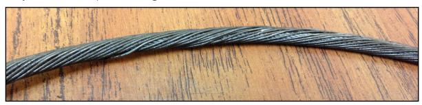
The picture shown below is from a crossed armor wire getting squeezed through a flow tube. The crossing of the armor wire probably occurred during re-heading and the crossed wire travelled all the way up to the flow tube and got jammed and broke.
