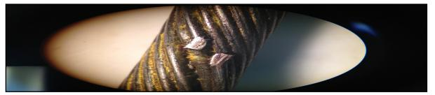
In the picture shown below it can be seen that the armor wires have been smashed due to heavy impact causing them to break.
