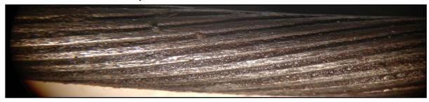
Another effect of damage due to loose armor can be seen in the picture below. This damage was most likely caused when it passed through the flow tube.
